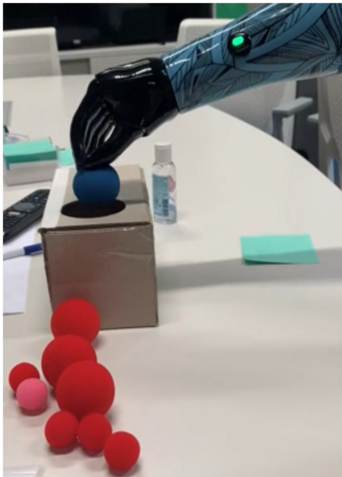
Figure 11: Some examples of the first skills of using a russian bionic below elbow prosthesis of the "Motorica"
